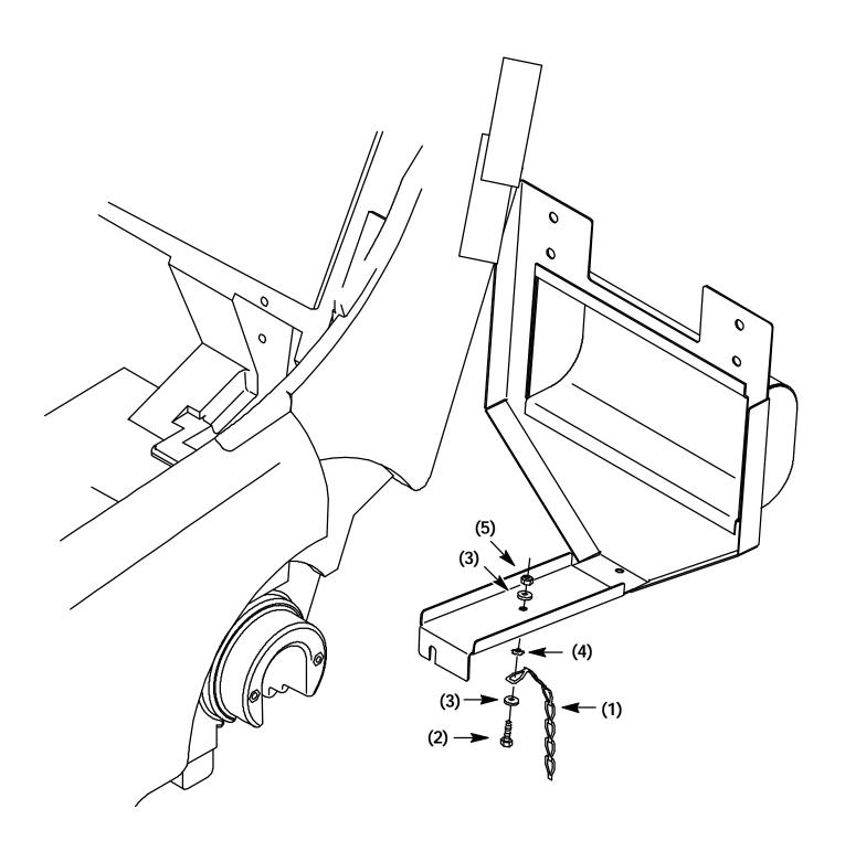
FIG. 1 - Chain And Hardware Assembly
