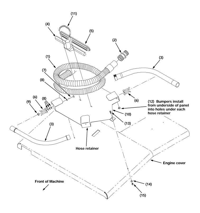
FIG. 1 - Installation of Vacuum Wand onto Engine Cover
