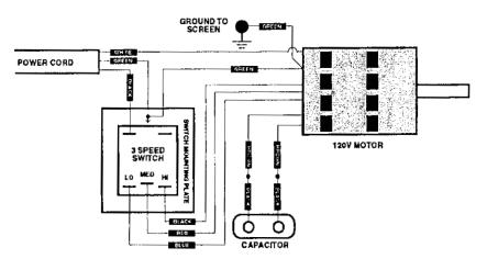
WARNING!!! To prevent shock hazard and seroius personal injury, connect the green grounding wires to the screen and to the switchplate as shown here.
