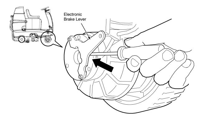
**FOR SAFETY:** After removing machine from crate, immediately remove screwdriver. Do not push, tow or park machine on an incline or operate machine when brake is disengaged.
