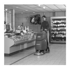
3.5 Setup the ec-H2O enabled machine for use at customer site. Run the ec-H2O machine for 10 minutes so that it calibrates the ecH2O system to the customer site. Make sure to run the machine in an area *away from any of the test sites*.
