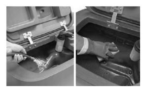
3.4 Before testing, clean out the recovery tanks of both the customer's existing scrubber, and the ec-H2O enabled scrubber. Make sure to completely clean out and drain the recovery-tank drain hose on both machines.
