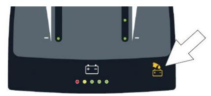
**NOTE:** To protect the batteries from damage, the machine's scrub function will be disabled after 10 hours of continued use if tank is not refilled. Add distilled water and restart key to clear the flashing indicator.
