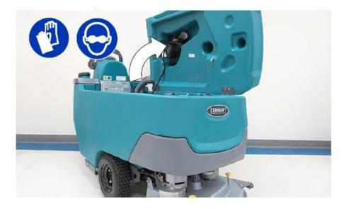
**C.** Remove the blue cap from the automatic battery watering tank. Using a funnel, fill tank with distilled water.
