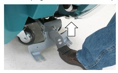
**B.** Mount the squeegee assembly to the squeegee mount bracket. Tighten the two inside yellow knobs to secure squeegee assembly to bracket.
