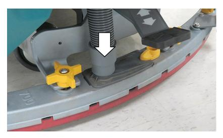
**D.** Check squeegee blade for proper deflection. Lower squeegee to floor and propel machine forward for a short distance. The rear blade should deflect evenly across the full length of the squeegee as shown. Refer to the Operator Manual for adjustment instructions.
