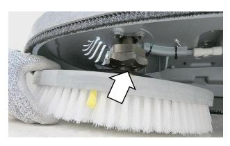
**C.** To remove the brushes, raise scrub head and step on the yellow brush release plunger.
