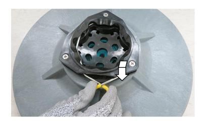
**B.** Align the brush under the motor hub and push it upward to engage hub. Make sure brushes are securely engaged.
