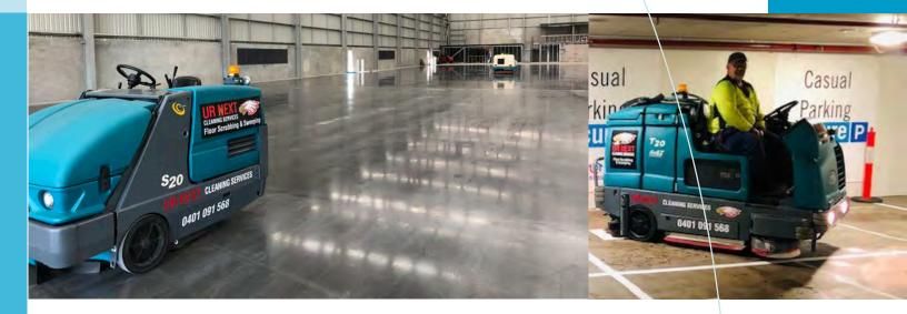
The reason for having a broad range of machines, especially the sweeper-scrubber combinations like the M30 & M20 works best when there is a site that needs sweeping and scrubbing immediately after one another. It is much more efficient to move one machine rather than the two. It also means that multiple jobs can be completed at one time.
