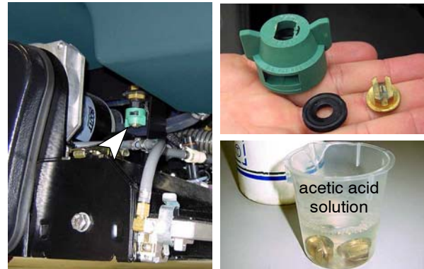
ReadySpace Spray Nozzle GREEN CAP / TIP #11002 p/n 575283000
